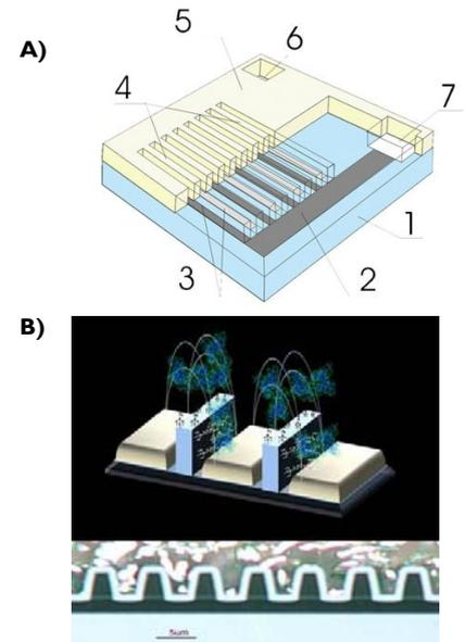
A) Interdigitated electrode array as biosensor transducer: (1) insulating substrate (2) electrode collector bar, (3) electrode digits, (4)  $\text{SiO}_2$  barriers between the electrode digits, (5)  $\text{SiO}_2$  layer and (6 and 7) aluminum contact pads. B) Insulating barrier with biomolecules immobilized in its surface.
